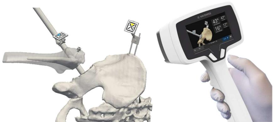
Fig 1: M-tag attached to the cup impactor for cup navigation (inclination, anteversion)
